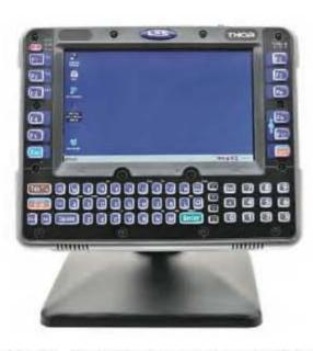
The Thor VM1 has a footprint of 10.6 x 8.4 inches-about like a netbook— and is around two inches thick. It weighs about 5.5 pounds, a bit hefty if you were to carry it around, but in line for a ruggedized vehicle-mount tablet. The Thor's resistive touch display measures eight inches diagonally and offers WVGA 800 x 480 pixel
